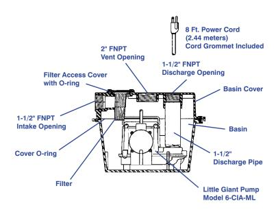
The compact "DRAINOSAUR" removes water from laundry trays, lavatory sinks, wet bar sinks, dehumidifiers, air conditioners (condensate), water softeners, etc. Installs above floor, no need to dig a sump. Unit is pre-assembled and ready-to-install.
